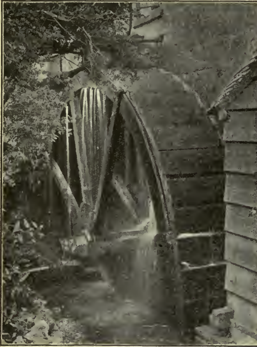
FIG. 48.—An old-fashioned water wheel used to furnish power for grinding grain into flour in a grist mill.
